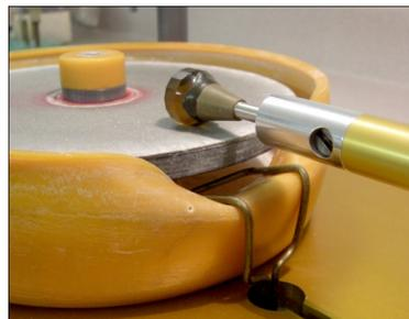
The bottom hook of the wire inserts through the keyhole in the Facetron base, anchoring the claw against the upward flex of the splash pan. The Ultra Tec instrument has this sort of convenience built-in (silver hook on the right of this image):
