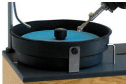
**The spill-proof swarf-catcher:** Swarf is slurry of ground gem material and water. Some of this stuff can stain some flooring, and all of it will leave behind a concrete-like residue if spilled. And, this isn't only an aesthetic issue, as gem swarf is micro-sized silica dust that can be very hazardous to your health, especially after it dries-up and becomes airborne. To protect your floor (and lungs), you can use a gallon (or larger) receptacle with a special cap.
