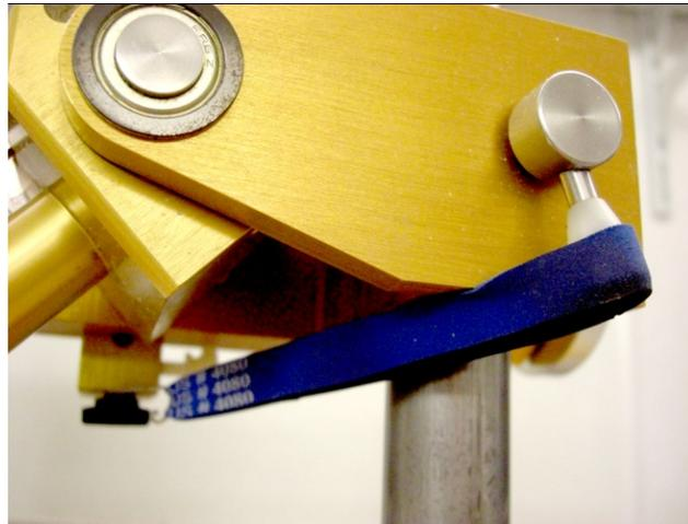
**DIY splash pan claw:** When doing girdle work on a large or troublesome stone - or using the dial indicator for precision dopping work ("lamp at the lap" technique), it's nice to work without holding the splash pan lip out of the way the whole time.
