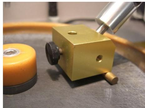
6. If the dial indicator still reads 0, then the indicator is calibrated. If not, then follow the dial calibration procedure that follows to set it. The procedure given uses the Facetron as an example. Details will vary from instrument to instrument. Consult your owner's manual or your manufacturer before adjusting your instrument!
