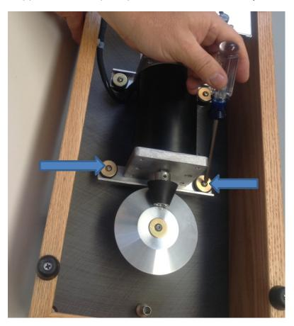
the rubber Drive Cone against the aluminum Driven Disc has to be increased. To get to the torque-adjustment feature, set the Base onto it's back-facing edge, allowing access to the bottom of the Base plate, where the Motor is mounted. With a screwdriver, very gradually tighten the two *forward* Motor Mounting Screws (see the two blue arrows). Balance the tightening between the two screws rotate the screws in small increments.
