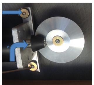
lift the front of the motor – providing space for the Drive Cone to pull away from the Driven Disk – allowing the Drive Cone to be pulled forward, and off the shaft.
