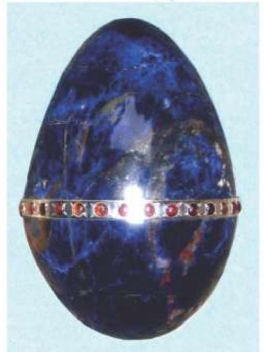
The outer ring was made to accept setting recesses 5mm diameter x 0.05mm deep for 32 cabochon stones around its circumference. These were machined by using the lathe headstock gearing as a dividing head and plunging a 5mm end mill in an electric drill clamped in the lathe toolholder, thus giving accurate pitching of the indents. At this stage I was beginning to tire and felt that I had bitten off more than I could chew - press on!
